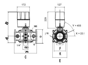
NOTES: The VE5065A/C has 4 flange holes instead of 8;  $Y = 90^{\circ}$ ,  $X = 45^{\circ}$
